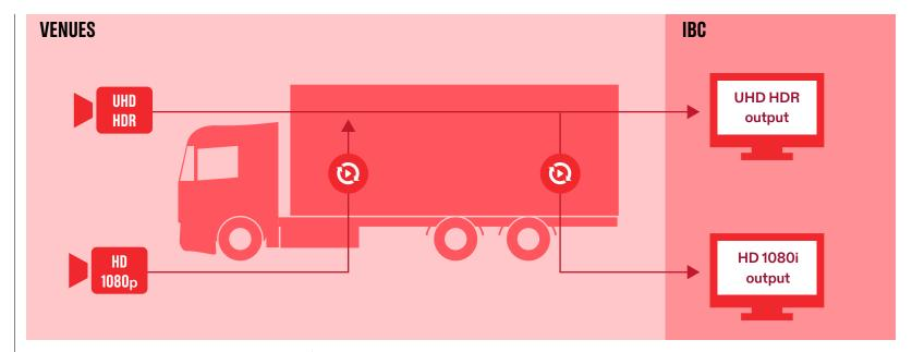
All RHBs will receive the output in HD 1080i SDR as per Olympic standards. OBS has created a single HDR to SDR production workflow model that will allow the trucks to generate an HD 1080i output via high-quality conversion from the primary UHD HDR signal.
